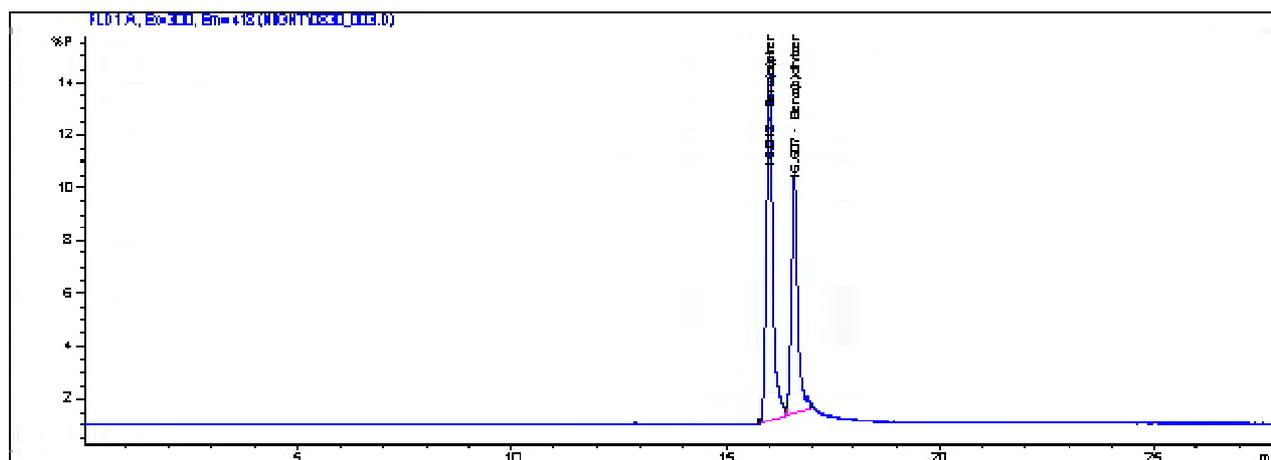
**Fig.1** HPLC/fluorescence detector chromatogram of benzo[a]pyrene and benzo[b]chrysene (1.0 µg /ml) standard solution
