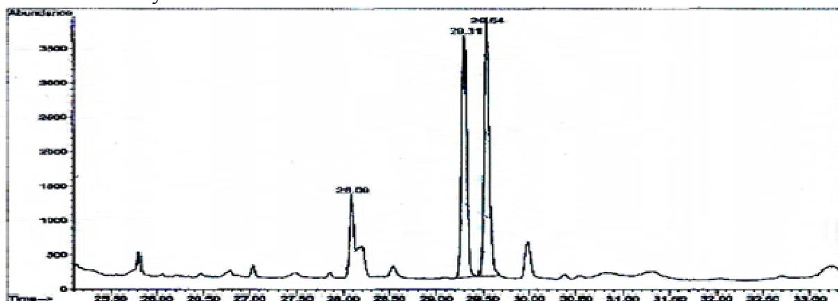
**Fig.2** GC-MS chromatogram of N,N-dimethylformamide containing benzo[a]pyrene and other PAH
